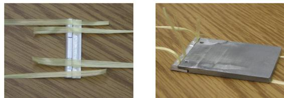
Figure 12: Demonstration of clamping method used to secure the Kevlar fibers
