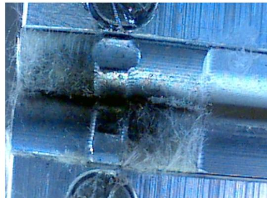
Figure 15: Abrasion of Kevlar fibers due to Aluminum Oxide
