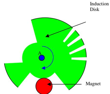
Figure 12: A non-uniform timing electromagnetic revolving cam
