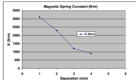
Figure 1: Magnetic Spring Constant 1cmx1cmx1cm magnets arranged to repel each other
