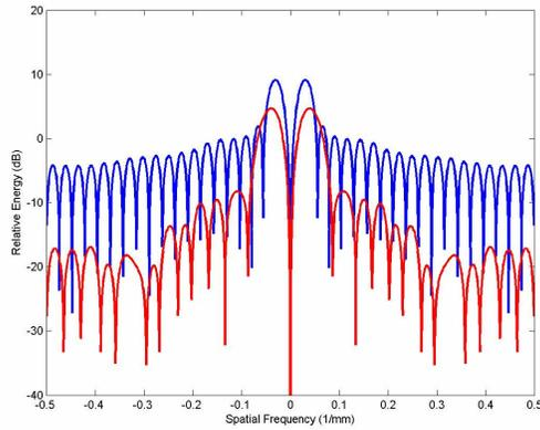
Figure 6: (a) Energy Well and (b) Fourier Spectrum. Red is for repulsive and Blue for attractive forces
