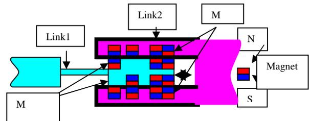
Figure 9: Prismatic Pair enhanced with magnets and/or dissipative members
