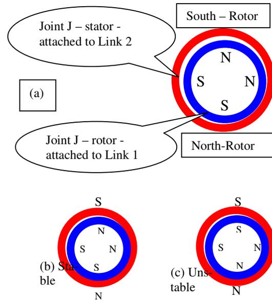
Figure 4: Electromagnetic interactions confined to the joints – Enhanced Revolute Pair
