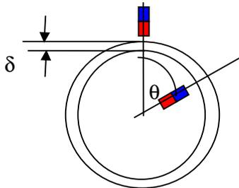
Figure 7: Torque produced by magnets
