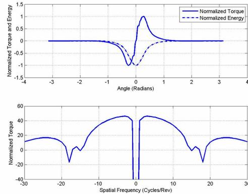
Figure 8: Torque and Energy for pole pair vs angular Separation (a) Torque/Energy versus angle (b) Spatial Spectrum of Torque (dB).
