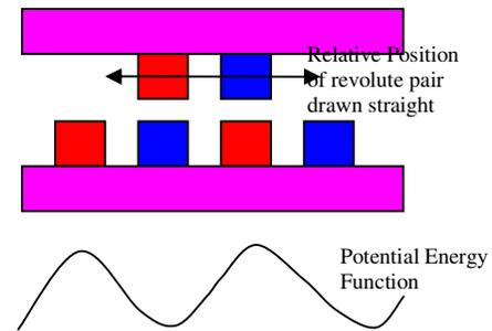
Figure 5: Energy Function of Revolute Pair drawn straight with rectangular poles.
