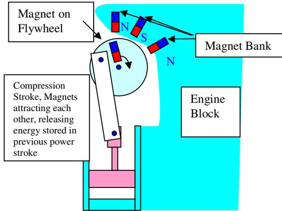
Figure 13: Engine (simplified sketch) with Flywheel and Block enhanced with Magnets, permitting storage of engine power magnetically.
