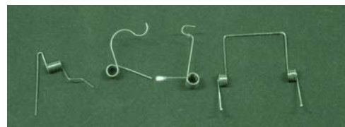
Figure 13: Different torsional springs used at the joints in the mechanism. These springs were cut and bent as needed in some cases.
