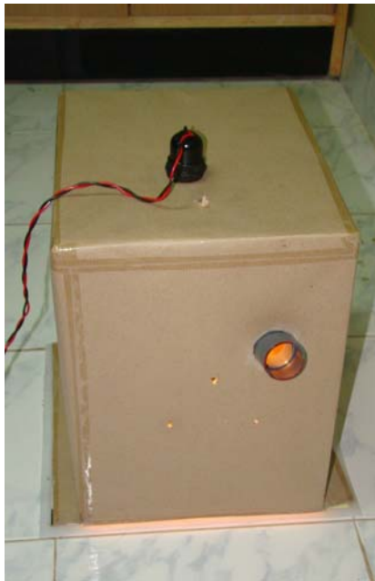
Figure 19: The set-up of a cardboard box with interior illumination, cameras for viewing the interior, and a hole for inserting a laparoscopic tool.
