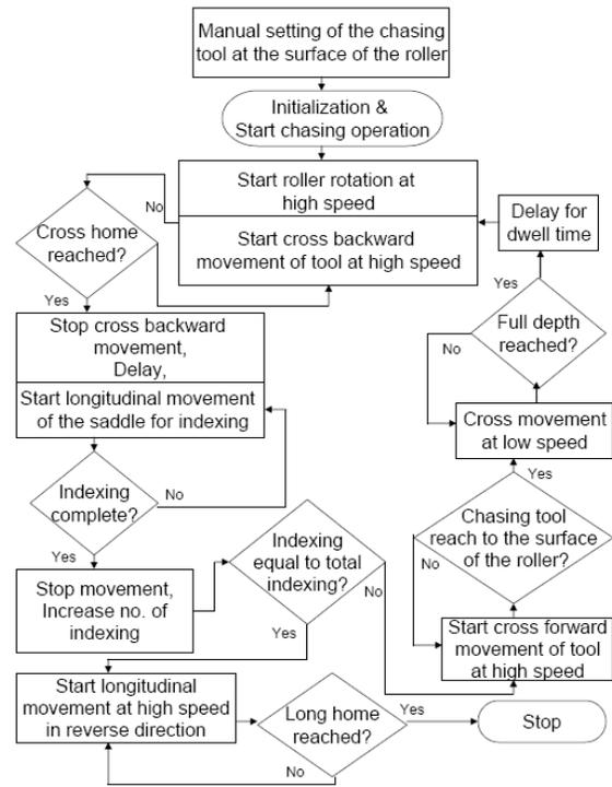
Fig.4: Flowchart of Chasing Operation
