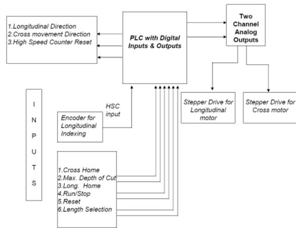
Fig. 3: Block Diagram of Electronic Controller
