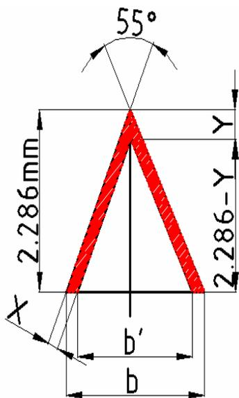
Figure 2:- chaser tool chip cross section
