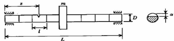
Figure 1: A finite element model of the rotor
