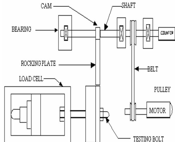
Figure 1: Schematic diagram of Testing Machine
