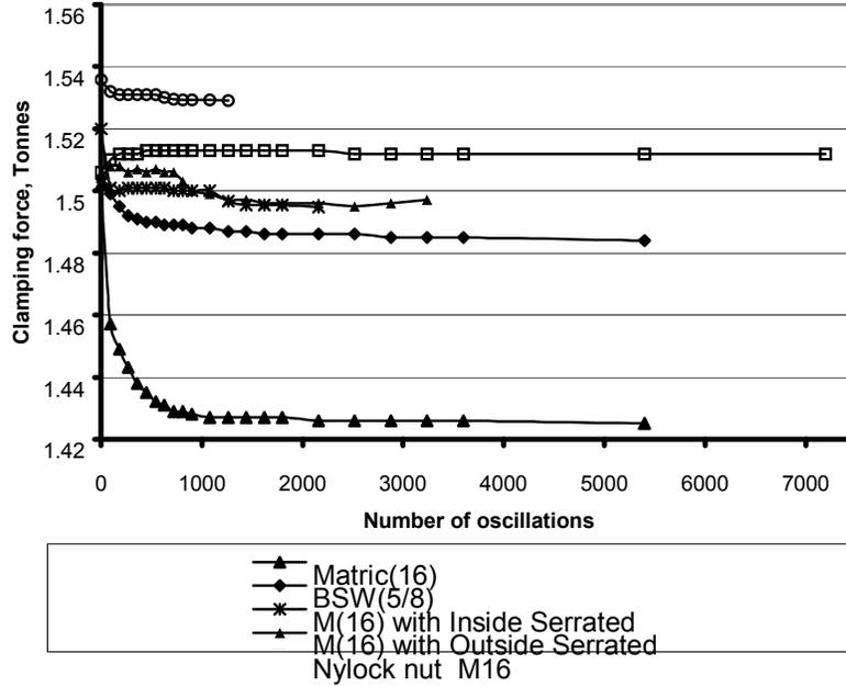
Figure 2: Loosening characteristics of fasteners with about 1.50 tonne clamping force
