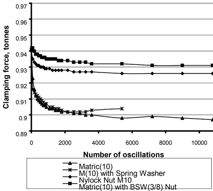
Figure 3: Loosening characteristics of fasteners with about 0.94 tonne clamping force
