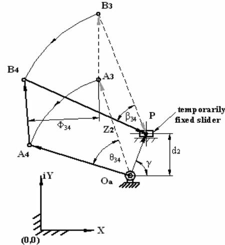
Figure 3: Off-set Five-bar slider mechanism with variable topology in phase-II
