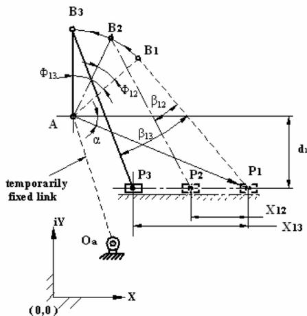
Figure 2: Off-set Five-bar slider mechanism with variable topology in phase-I
