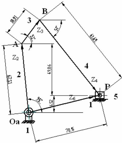
Figure 5: Synthesized off-set Five Slider Mechanism with variable topology for the example 2
