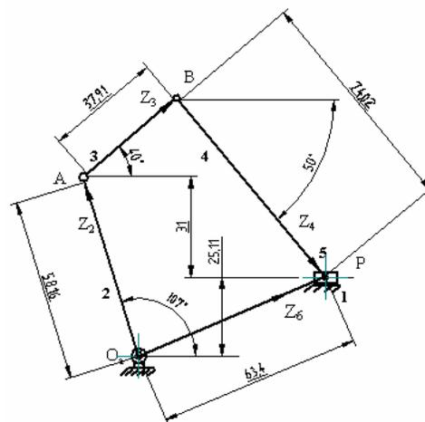
Figure 4: Synthesized off-set Five Slider Mechanism with variable topology for the example 1
