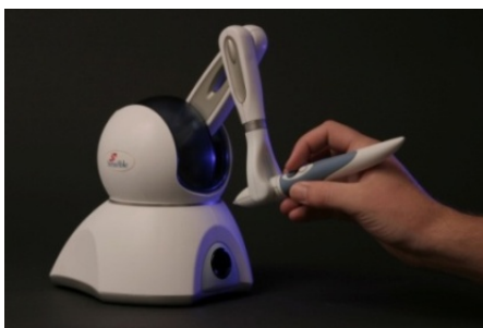
Figure 4: The Phantom Omni haptic interface device by Sensable Technologies. (Courtesy: Phantom manual from Sensable Inc.)
