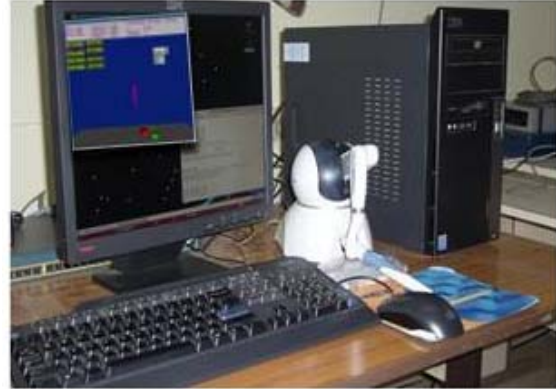
Figure 10: Test set-up showing Phantom Omni haptic interface device connected to the simulation system.
