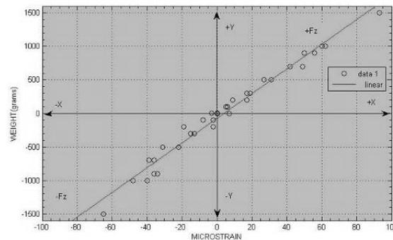
Fig. 7c Strain variation in Leg1 for  $F_z$
