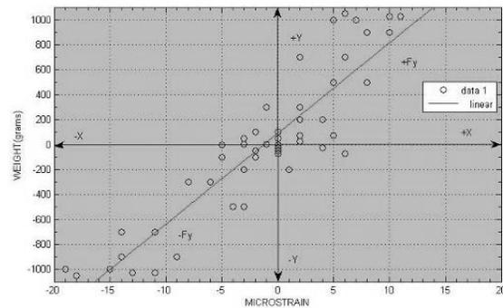
Fig. 7b Strain variation in Leg1 for  $F_y$
