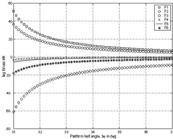
Fig 1b – Leg force variations in a configuration close to singular configuration
