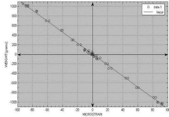
Fig. 7a Strain variation in Leg1 for  $F_x$
