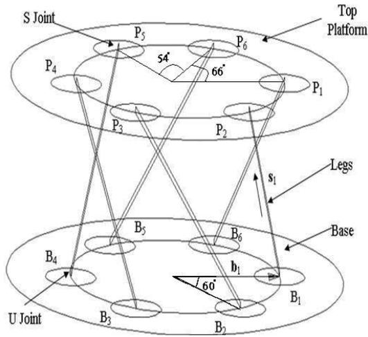
Fig 1a – Line diagram of a 6-6 Stewart platform based Sensor
