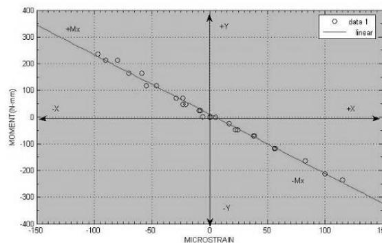
Fig. 7d Strain variation in Leg1 for  $M_x$
