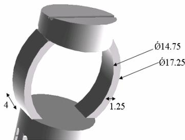
Fig 4 – Ring sensing element
