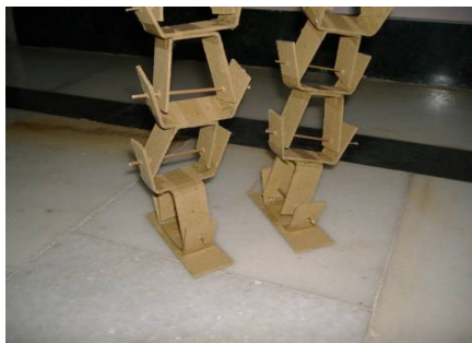
Figure 5: Proto type model made from card board. By using this model individual joint movements are studied.
