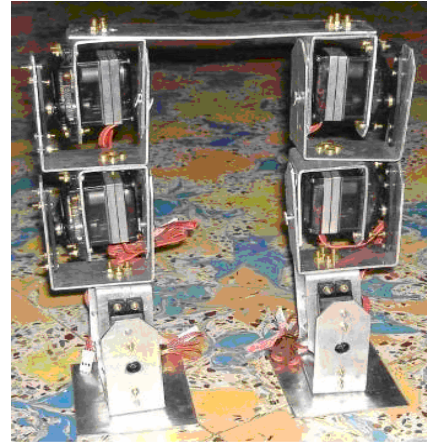
Figure 6: Fabricated Model. It has been made from 1.5mm aluminium sheet.
